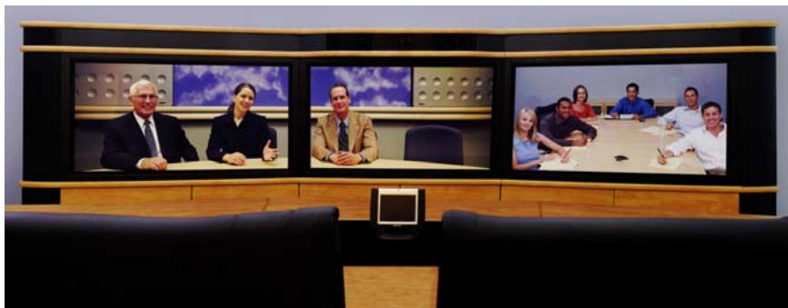
Figure 5. A Polycom immersive telepresence system, video solution with group system integration (right screen).
