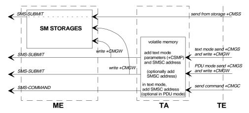
Figure 4: Message service send and write procedures
